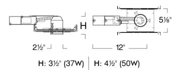
5 1/2" minimum clearance above ceiling recommended for installation and maintenance access. Can be used for remodel applications as well.
